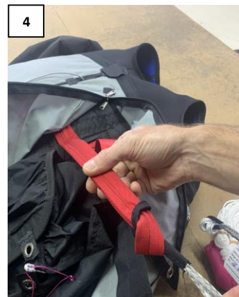
Tie the parachute bridle to the security webbing. Certify that the tie is correct
