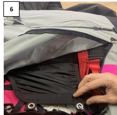
Use the thin rope as a guide to pass the rubber band through the first eyelet.
